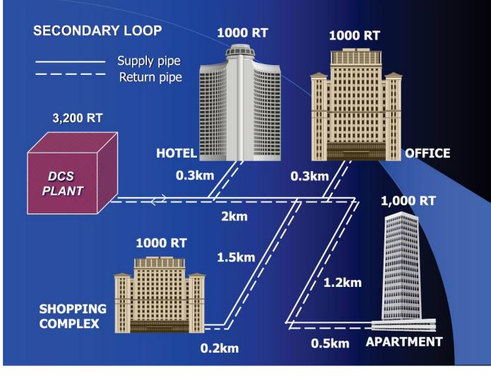
District cooling is the production and distribution of chilled water from a central source to facilitate air conditioning. This is done by producing chilled water at a central plant and then piping the water to customers through an underground insulated pipes network.\*
